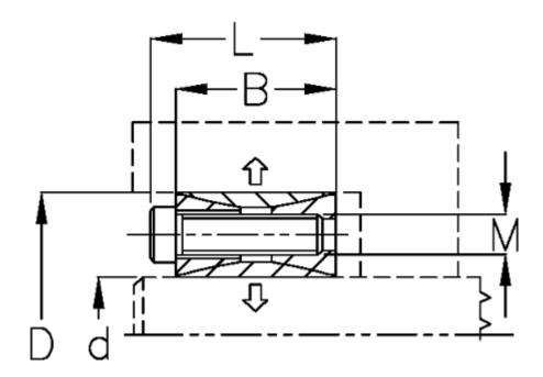
$\begin{array}{lll} {\rm B} \ {\rm mm} & = 24 \\ {\rm d} \ {\rm H8} \ {\rm mm} & = 5080 \\ {\rm D} \ {\rm mm} & = 80 \\ {\rm Fit} \ {\rm tolerance} & = {\rm Aksel} \ {\rm k11-h11}, \ {\rm Nav} \ {\rm N11-H11} \\ {\rm F} \ {\rm kN} \ {\rm torque} & = 80.0 \end{array}$
